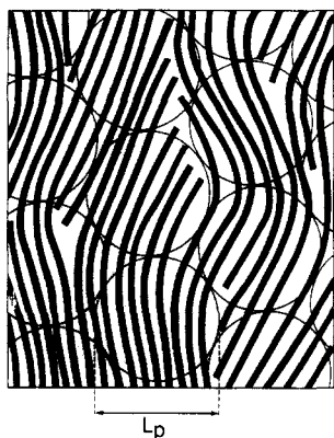
Figure 11. Schematic structure in a lyotropic phase with "blobs of dimension L_p ".
